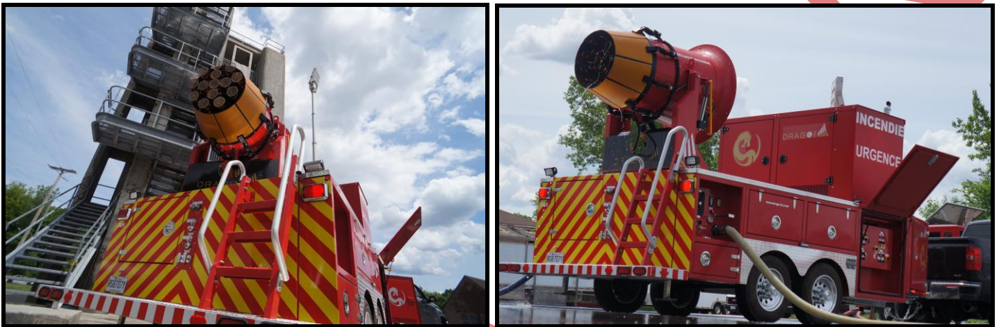
Fig.2 Spider nozzles system (Foam and water)
