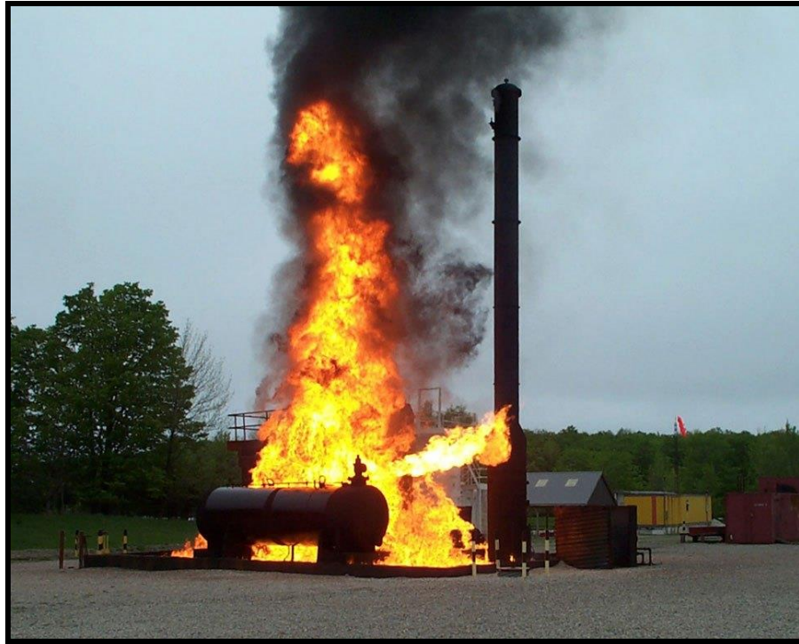
Fig. 4 - 3D B class test rig
